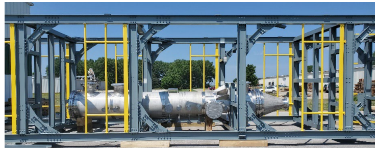
Completed pyrolysis reactor module
